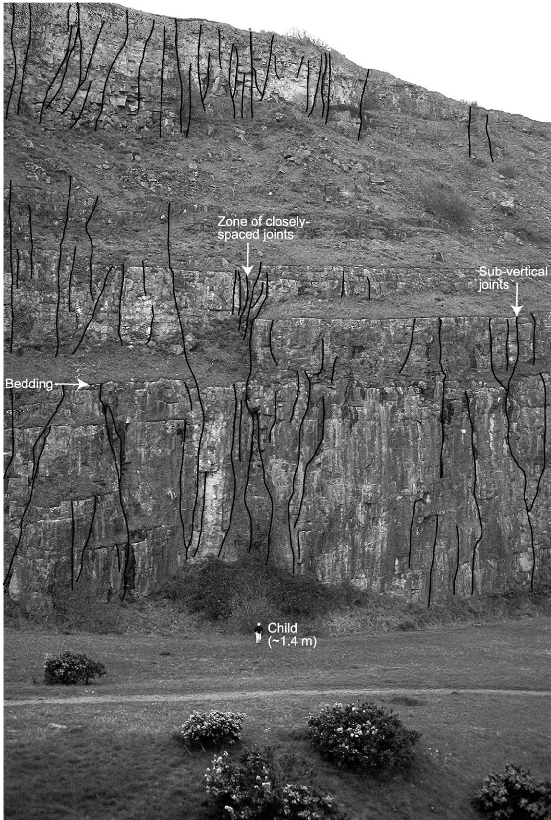
Fig. 1. Photograph of gently dipping Carboniferous Limestone and sub-vertical joints (highlighted in black), Colwyn Bay, North Wales. Zones of relatively closely spaced joints occur in the cliff, illustrating how different numbers of joints can be intersected by wells that are a short distance apart. A deviated well with an azimuth at a high angle to the strike of the joints would give a better measure of the joint distribution through the rock mass than would vertical wells.
